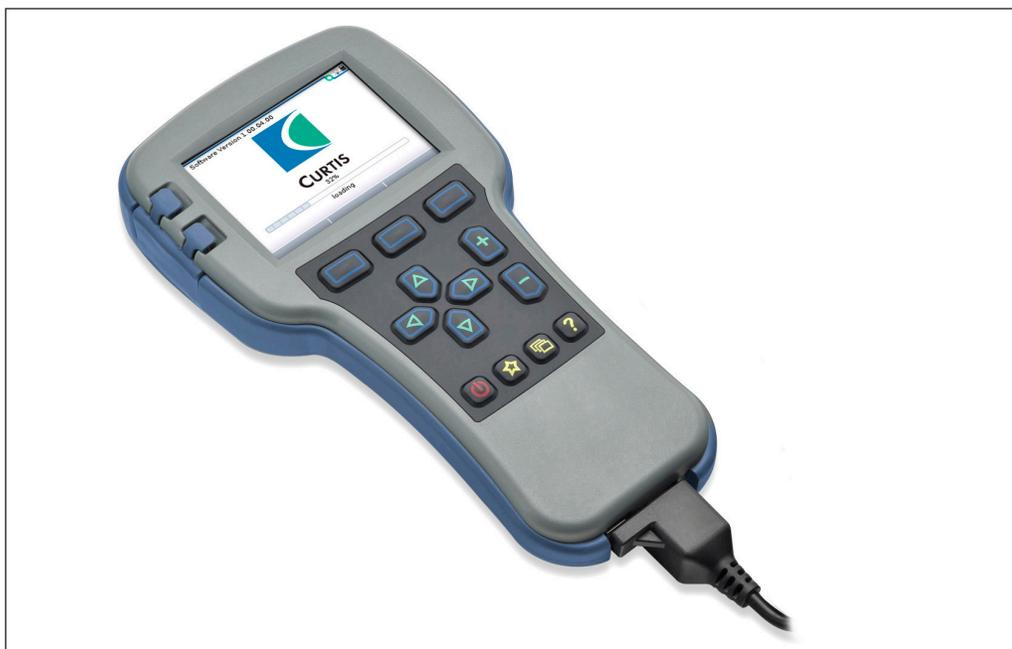
**This manual covers the operation for the Serial-connected programmable controllers. Gauges and control systems (devices) operate in a similar fashion.**
