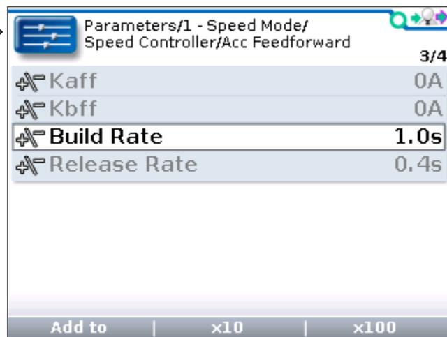
Note that when the Speed Mode folder is highlighted, the “x10” and “x100” softkeys are grayed out (indicating they do not apply)—but when Build Rate is highlighted, these softkeys are available.
