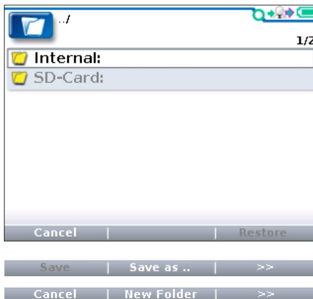
“[Save as ..](#)” The “Save as ..” softkey saves the .cpf file to the current location using the name from the pop-up keyboard (see [Chapter 13](#), Using the Keyboard). The default name is based upon the ‘Text for “save as”’ setting in the HHP Settings app.
