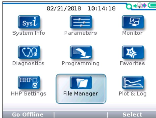
In the main screen, highlight the File Manager icon and press the “Select” softkey to enter the app. Return to the main screen at any time by pressing the main screen key (⏏).
