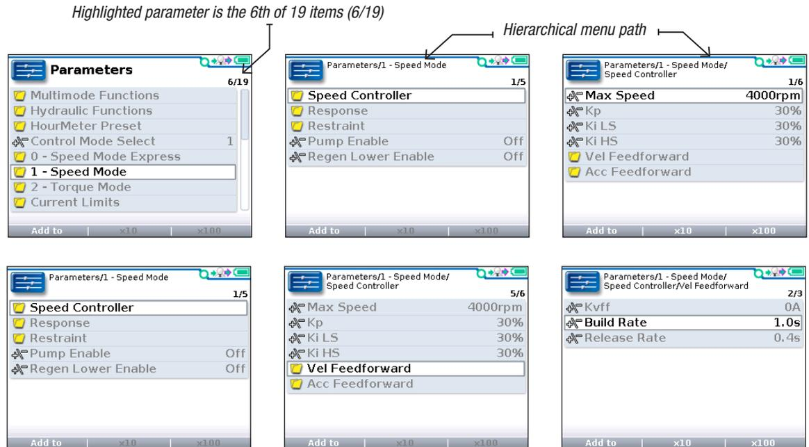
If exiting an app using the main screen key (⏪) and later returning to the same app, the app will open to a location that depends on the “Remember Last View” setting in the HHP Settings app. If the “Remember Last View” setting is “Off”, the app opens at the top-level. If the setting is “On”, the app opens to the most recently used location.
