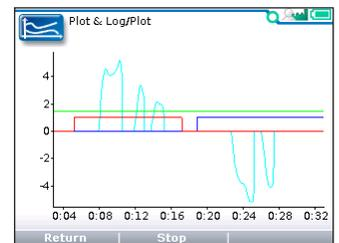
Plot variables versus time: Use the softkeys to **Select Plot**, **Start the Plot**, **Stop** when complete, and then **Save** the file to the SD card.
