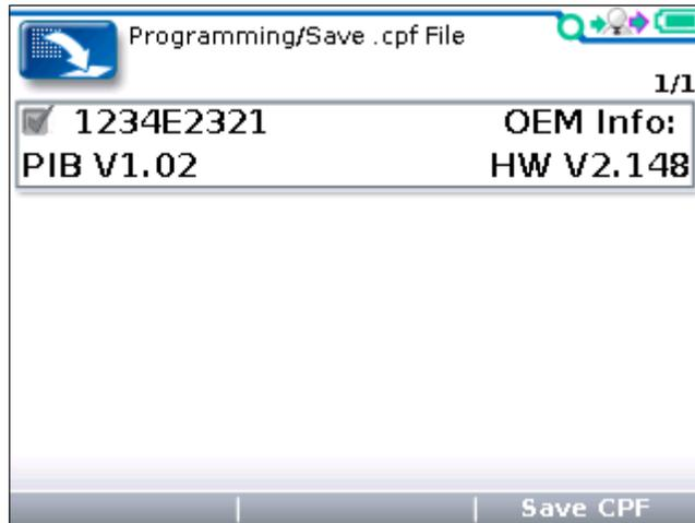
Pressing the “save CPF” softkey will confirm the controller-model from which the data will be saved. In some applications, several modules (controllers) can be listed. In these cases, highlight the desired module.
