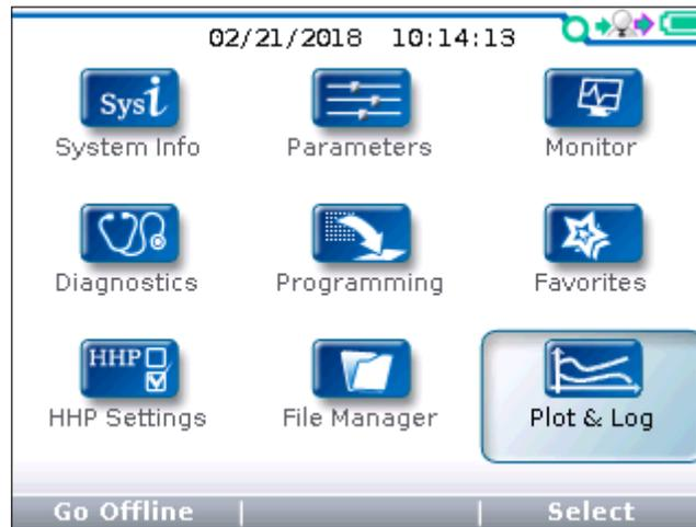
In the main screen, highlight the Plot & Log icon and press the “Select” softkey to open the app. The Plot & Log app has a Plot utility and a Log utility. The Plot utility plots the values of selected variables over time. The plot can be saved using the screenshot process. The Log utility creates a log of the values of selected variables over time. The log can then be viewed in a spreadsheet program on a PC. Return to the main screen at any time by pressing the main screen key (⏪).
