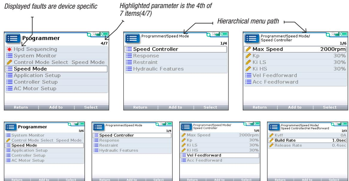
If exiting an app using the main screen key (⏏) and later returning to the same app, the app will open to a location that depends on the “Remember Last View” setting in the HHP Setup app. If the setting is “Off”, the app opens at the top-level. If the setting is “On”, the app opens to the most recently used location.
