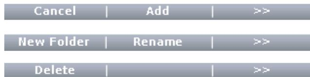
The “Add” softkey adds the new item to the Favorites main window. The “Cancel” stops the operation and returns the screen back to the highlight item in Parameters or Monitor. Use the “»” softkey to scroll to the other softkey options.
