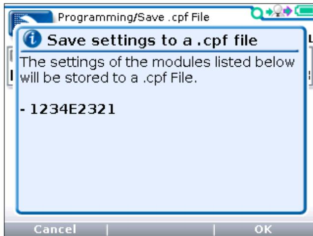
After pressing “OK” to proceed in saving a .cpf file, the 1313 HHP will open a screen to select the location to save the file. Select either the Internal or SD-Card. Based upon the “Remember Last View” setting (see [Chapter 10](#), HHP Settings app) or if a .cpf file was previously saved, the next screen will vary.
