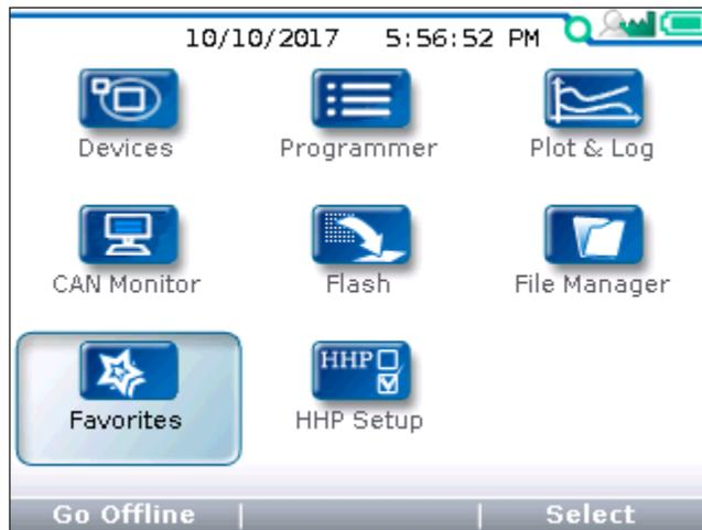
In the main screen, highlight the Favorites icon and press the “Select” softkey to enter the app. Alternatively, the Favorites key (★) opens the app directly. Return to the main screen at any time by pressing the main screen key (☐).
