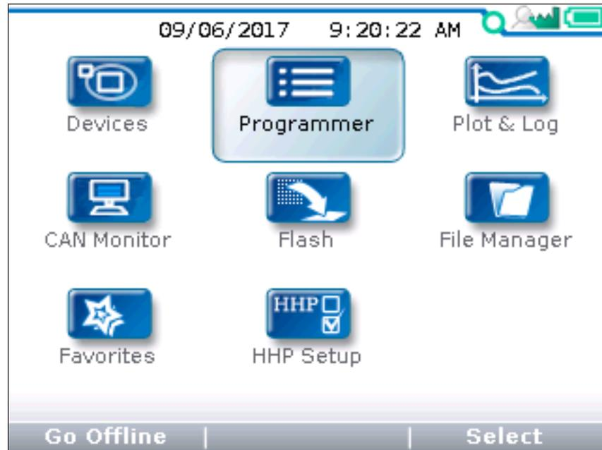
To select an app, scroll using the arrow keys (⬆️) until the app is highlighted. Apps can also be selected by successive presses of the main screen key (⏏). Each press will highlight the next app.
