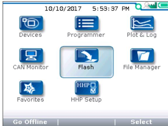
Use the Flash app to obtain and save parameter values, restore (load) parameter values to the device, or update the device’s firmware. Highlight the Flash icon and press the “Select” softkey to open the app.
