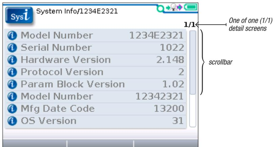
The sliding bar at the right of the screen indicates there are more items than those shown. Use the down-arrow key (⏴) to scroll down to see the rest of the list.
