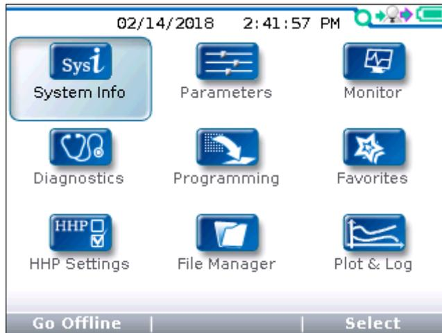
After the 1313 HHP powers up and loads the controller information, the Main Screen is displayed with the System Info app highlighted. The System Info app is where the controller-specific information is viewed. Press the “Select” softkey to view information such as the controller model number, serial number, manufacture date, and its software/firmware/hardware versions.
