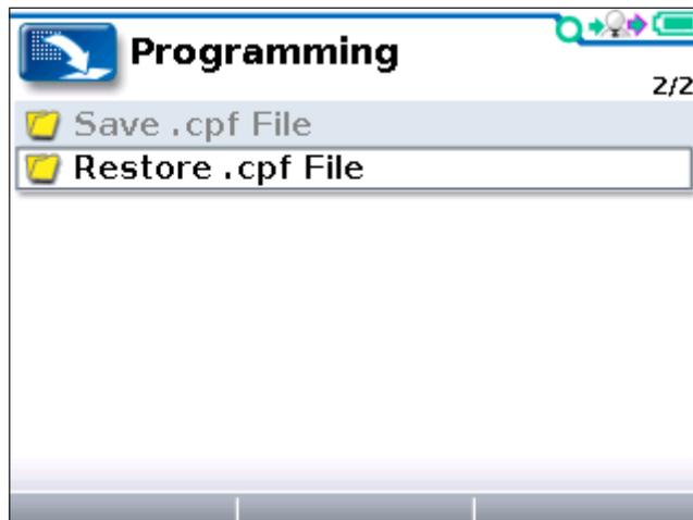
There are no softkeys on this screen. To choose whether to Save or Restore a .cpf file, highlight the option and press the right-arrow key (→).
