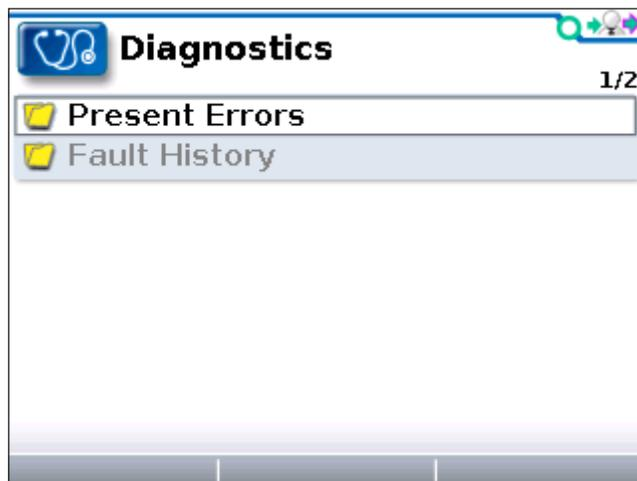
Note: Sometimes the fault circuits catch a temporary event that is not a true fault in the system; it is always a good idea to turn the control system off and back on again to see whether the fault clears by itself.
