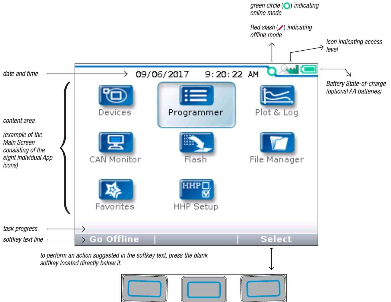
In this above example, pressing the “Select” softkey will open the highlighted Programmer app. The “Select” softkey opens whichever app is highlighted. Pressing the "Offline" softkey switches the 1313 HHP to Offline mode. In Offline Mode, the 1313 HHP cannot communicate with the device. The 1313 HHP can perform operations that do not require communication with the device. [See Chapter 14.](#)
