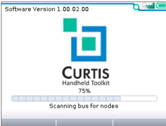
(1) 1313 HHP startup-scan of CANbus for devices
