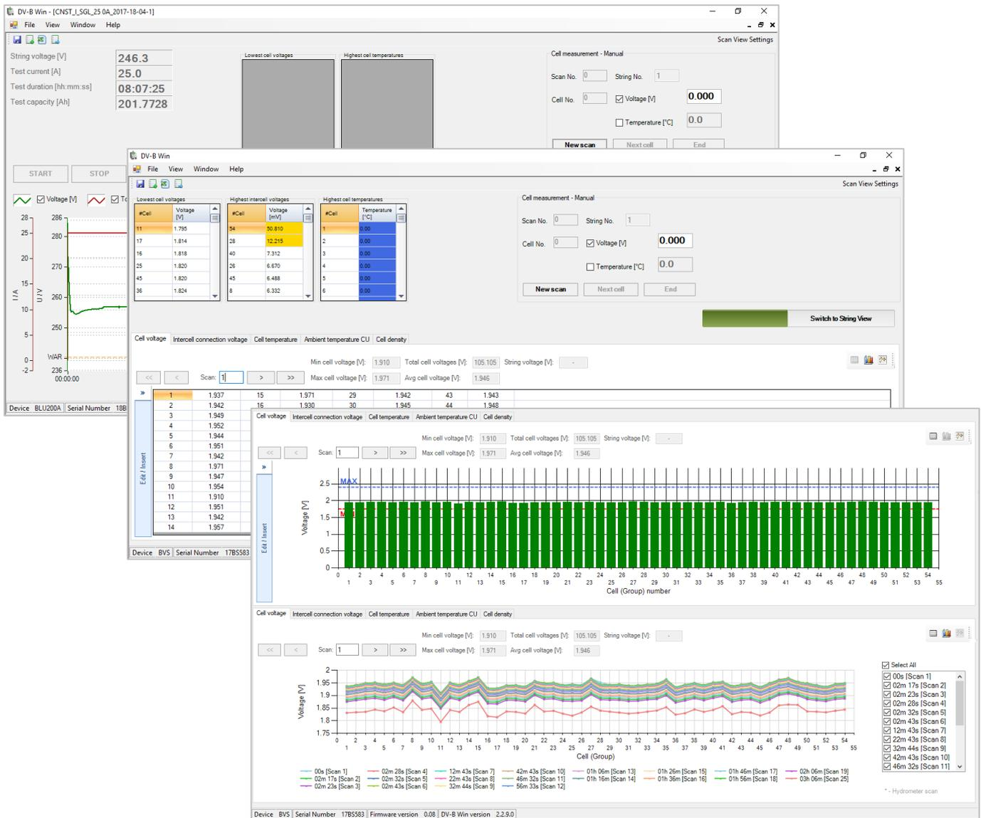
DV-B Win application functions – string view, battery scan view and line voltage chart
