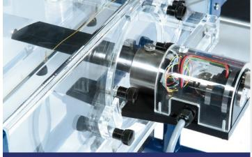
A 2-component, electronic balance used to measure the lift and drag on appropriate models. The lift and drag models connect to the balance using a simple fixing that ensures correct orientation of the model.
