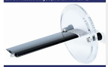
A symmetrical aerofoil incorporating 10 tapping points distributed along the wing profile on one side, which allows the pressure distribution to be measured from the leading edge to the trailing edge.
