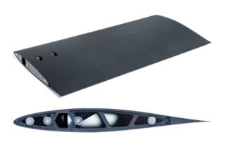
Wing model designed with a NACA 64-212 profile, as used on the MDM-1 Fox aerobatic glider. The profile is almost symmetrical and cuts through the air evenly.
