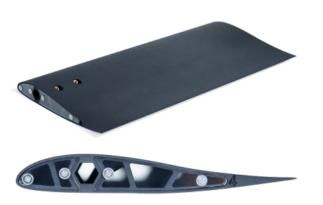
Wing model designed with a **Fauvel F2** as used on the FV-36 Flying Wing. The profile is a reflexed camber air foil where the camber line curves back up near the trailing edge. Such an air foil is useful in certain situations such as with tailless aircraft.
