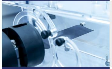
A 3-component balance used to measure lift, drag and moment forces on appropriate models.
