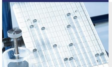
The bank of 13 transparent tubes inclined at 30° to measure small pressure differences (0-160mm H2O).
