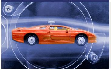
The probe smoke generator allows for easy visualisation of the air flow.
