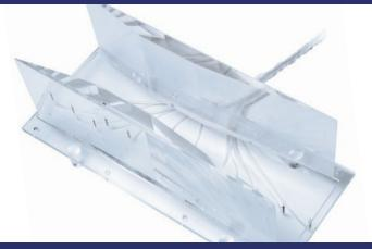
A Venturi profile that is installed in the working section of the tunnel via the removable floor. The Venturi incorporates 11 pressure tappings in the floor, connected via flexible tubing to quick release connectors.
