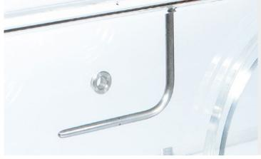
A miniature Pitot Static Tube mounted in a support plug that can be located in the roof of the working section at three alternative positions, i.e. the start of the working section and upstream and downstream of the model mounting position.
