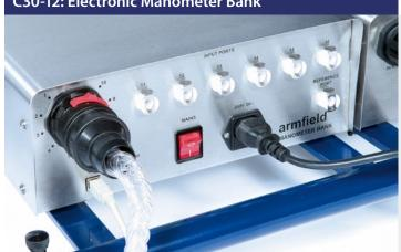
An electronic console incorporating 16 differential pressure sensors, each with a range of 0-178mm H2O.
