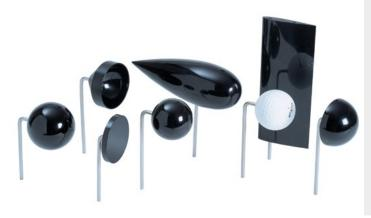
Seven different models are provided for use with the C30-13 Lift and Drag Balance for investigations into the influence of shape on the drag forces.
