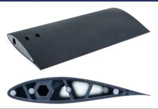
Wing model designed with a NACA 633-618 profile, as used on the Schleicher Ka6b Glider. The profile is less cambered than the Gottingen 535 allowing direct comparison.
