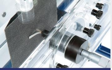
A flat plate, with a bevelled leading edge, that is mounted vertically in the working section via the removable floor. A flattened Pitot tube, mounted on a traversing micrometer, allows the air velocity to be measured at different distances from the surface of the plate.
