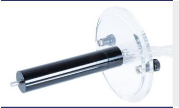
A plain cylinder, 30mm diameter, incorporating 10 equi-spaced tapping points around half of the circumference that allow the pressure distribution around the cylinder to be measured.
