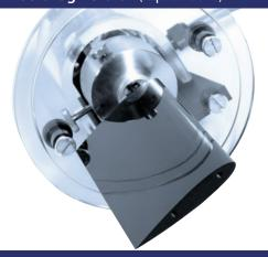
A plain symmetrical aerofoil to NACA 0015 profile, incorporating a mounting rod that allows it to be installed on the C30-13 Lift & Drag Balance, thus allowing the lift and drag to be measured with the aerofoil at different angles of attack.
