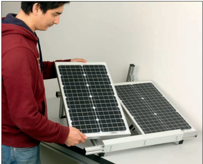
Panel frame mounting: roof installation simulation
