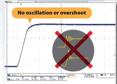
Output voltage waveform with 400 µF capacitor connected
