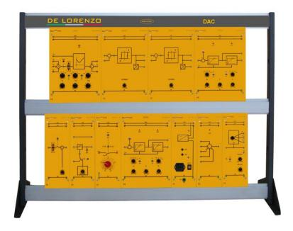
This laboratory is designed for the study of Discontinuous Automatic Control systems where the controller is composed of a an element with discontinuous intervention. A discontinuous controller is characterized by an output having two or more fixed states and its value is switched among these states according to the input value.
