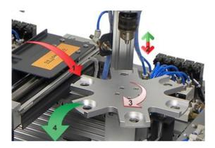
We study here an integrated motion system (motors, mechanical power transmission devices, encoders, sensors, and controllers). We underline the important parameters for rotary indexing tables (the needed resolution of the application, the required repeatability and accuracy, and other mechanical parameters such as acceptable levels of backlash or hysteresis).
