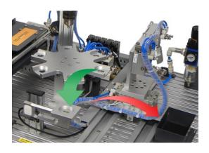
A simple and robust decision maker algorithm has been implemented in DL CIM-B based on the weight of the work pieces.
