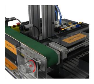
The **DL CIM-B** trainer offers an excellent possibility to study, understand, and design the most appropriate applications of a DC motor use (a). Simple, easy to control, with some proper gear, the application for belt conveyer is fast integration of this electric machine in manufacturing chain.
