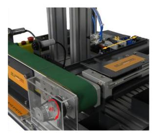
The **DL CIM-C** trainer offers an excellent possibility to study, understand, and design the most appropriate applications of a DC motor use (a). Simple, easy to control, with some proper gear, the application for belt conveyer is fast integration of this electric machine in manufacturing chain.
