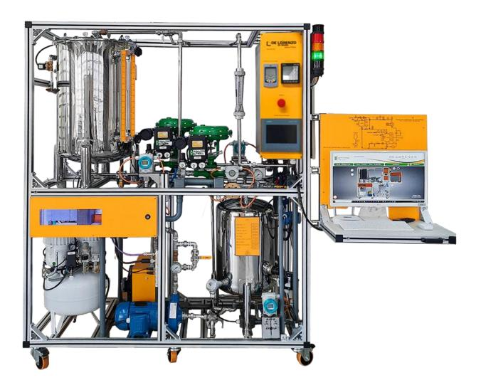
This pilot plant of theoretical and practical training offers the possibility to study the control in open loop and in closed loop of the four typical processes used in the industry: LEVEL / PRESSURE / TEMPERATURE / FLOW.
