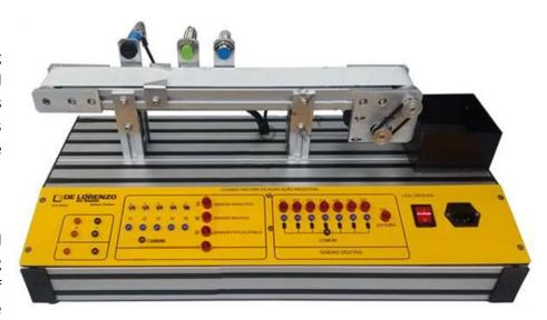
supplied and routed to a collection box. The pieces act on three types of sensors - normally used in automation — which are: One optical, one capacitive and one inductive, which by means of programming allow to separate and count, by type of material of the piece.
