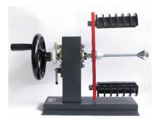
To be fixed to the bench, it allows the manual winding of motor coil or of linear windings without wire guide. Complete with a 300 mm diameter faceplate, a pair of square mandrels, a pair of 6 grooves straight arbors, 60 mm diameter, a central arbor for linear winding and a 5 digit revolution counter.
