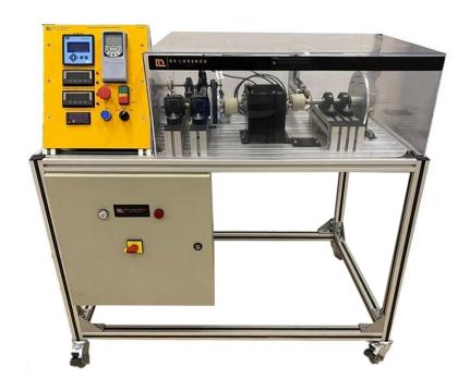
The system allows the evaluation, after each assembly and disassembly, of a set of shafts and bearings driven by belts, gears and toothed pulleys driven by a three-phase motor whose variable speed implies a higher or lower level of vibration; the vibratory intensity is measured on all three shafts.
