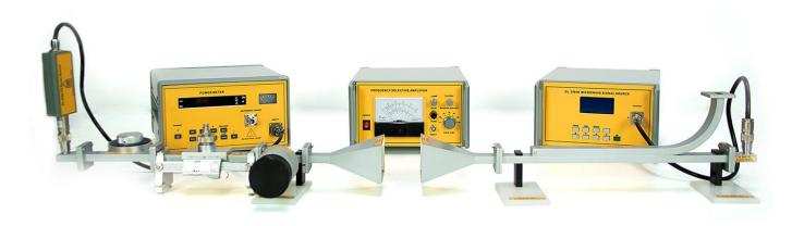
The trainer has been designed to introduce students to the microwave technology. It consists of a set of components, accessories and instruments and can be used as a laboratory test bench to experiment with the microwaves components as well as to study the aspects of wave propagation.
