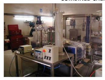
Our Chemical Reaction Plant allows the study of chemical reactions in a tubular chemical reactor and in a stirred tank reactor.
