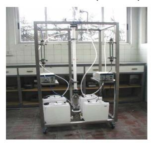
When the separation by distillation is ineffective or impractical, the liquid-liquid extraction is one of the alternatives to consider.
