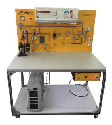
Didactic station for cooling, with split-type air conditioning of 9000 BTU/h, reverse cycle (hot/cold). An air conditioner is basically a cooler without its cabinet and its basic parts are the compressor and the coil. It uses the evaporation of a refrigerant fluid (the gas circulating in the coil) to provide cooling. The mechanisms of the cooling cycle are the same as those in an apartment's fridge and air conditioning. It uses a non-flammable gas compressed by a compressor.
