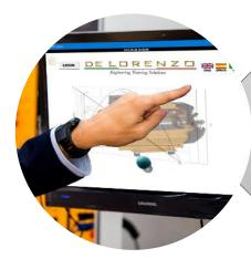
**Data acquisition software for electric machines**: performs the test automation and provides the user interface to execute the experiments. The SW developed in LabVIEW communicates with the acquisition devices via serial port using the Modbus protocol, reading electrical and mechanical data from instruments.
