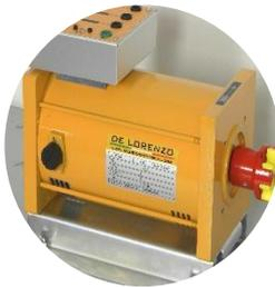
A DC motor is used as a prime mover for the study of AC and DC generators and the synchronization of machines with the mains network.
