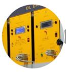
Multifunction digital modules to collect all the electrical parameters (voltage and current in AC and DC, RMS values, active, reactive and apparent power and frequency) and mechanical parameters (speed, torque) needed to characterize the machine under study.
