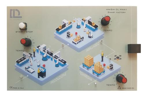
The DL MiniSim-MAN1 is used, which shows a screen print of the components of the complete system and shows the status of the different workstations through multi-colored LEDs.
