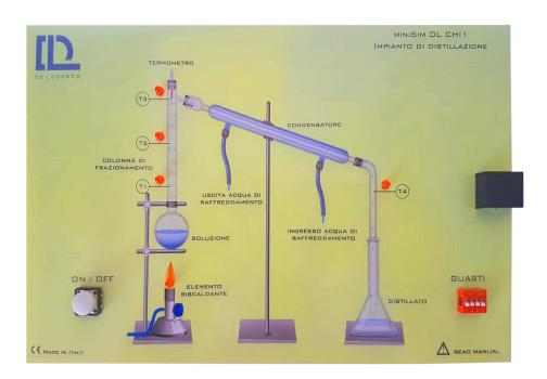
The DL MiniSim-CHI1 which shows a screen print of the distillation system in all its components, also contains a microcontroller inside which allows the simulation of the operation of the plant. During the simulation, all the values of the main physical magnitudes that characterize the system are calculated in real time.
