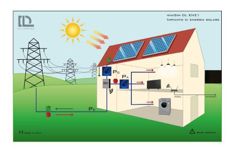
The simulator of the DL MiniSim-ENE1 solar system is used, which shows a screen print of the components of the domestic system, and allows to vary, through the potentiometer, the energy produced by the solar panels (to simulate different environmental conditions) and the energy absorbed by the domestic charges. The power absorbed or sent to the network operator is calculated with a subtraction.
