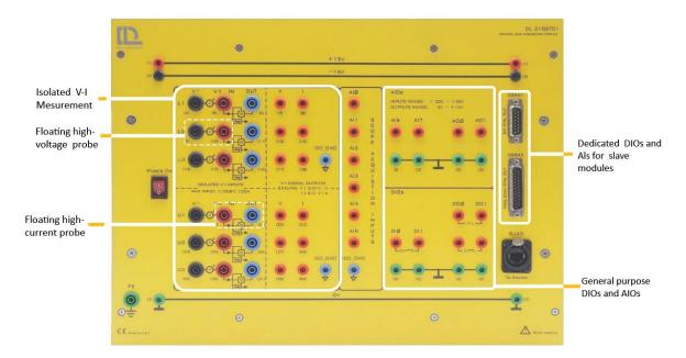
Maximum 9 signals of voltages and currents can be measured simultaneously. The signals connected to the front panel are well isolated from the controller for the purpose of reliability and anti-interference. It communicates with the control software via ethernet.
