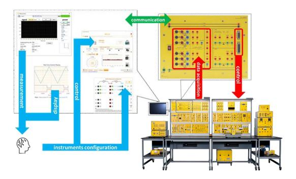
The software interface is programmed using LabVIEW, a language widely used in the industry and academy. The all-in-one user interface provides a clear view of signals being created to control the semiconductor devices and powerful visualization and mathematical tools to observe the resulting waveforms to study and simulate different controllers and power conversion strategies used in the industry.
