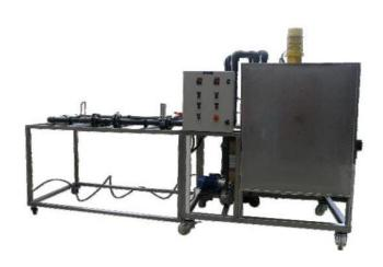
The Heat Exchangers trainer has been designed for the study of these devices that are extensively used in the industry. It is also possible to study the theory of the heat exchange, by measuring the temperatures at all points of interest, and to study the influence of different parameters on the effectiveness of the exchange.
