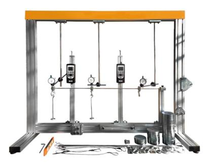
The modular training system **DL ST33** allows users to study theoretical-practical assemblies involving beams and gates, to measure with two electronic dynamometers and to visualize the applied force values graphically on PC (not included).
