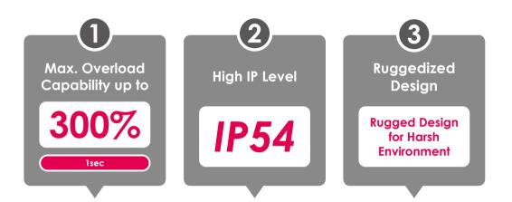
With the protection level up to IP 54, the AMV series is a ground power unit designed for outdoor usage. The overall design and main components have been ruggedized for harsh environments. For inductive type of DUT, such as motor or compressor, the AMV series has standard overload capability of 125%, 150% and 200%, and it is extensible up to 300%, which makes it suitable for DUT with high startup inrush current and can further reduce the cost on scaling up the power unit.
