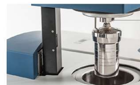
Automatic bomb raising & lowering Automatic oxygen filling & releasing
