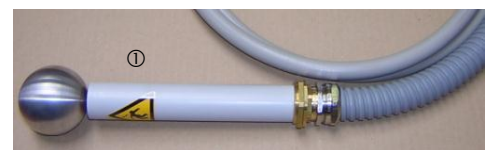
HIGH VOLTAGE OUTPUT ON HIGH VOLTAGE CABLE (first picture is the output from the transformer, second one the ending)
