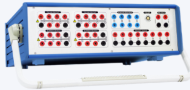
Traditional protection relay test set
