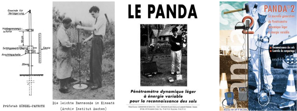
Figure 1. (a) Prüfstab Künzel-Paproth" (Menzenbach, 1959) (b) Panda@ lightweight dynamic variable energy penetrometer: first generation (Gourvès R. , 1991) and (c) Panda 2@: second generation.
