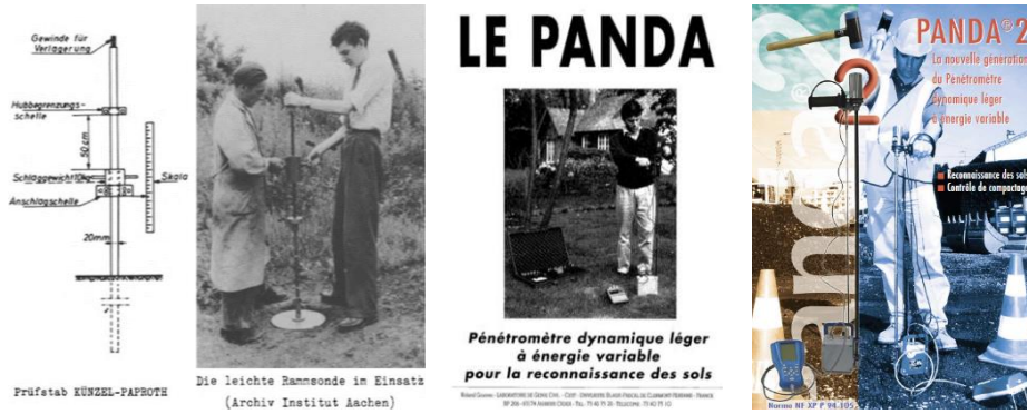
Figure 1. (a) Prüfstab Künzel-Paproth" [6] (b) Panda® lightweight dynamic variable energy penetrometer: first generation [7] and (c) Panda 2®: second generation.
