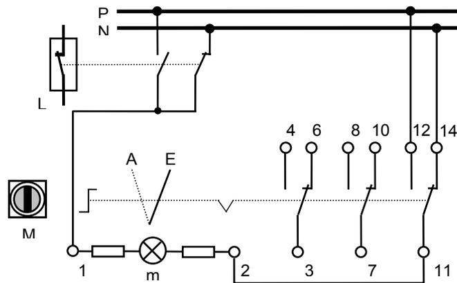
Rs 801 346 diagram of connection: Figure 2 – Switch L switched on, position acknowledged
