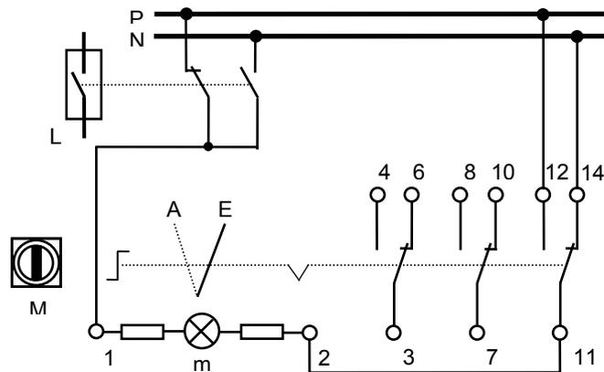
Rs 801 346 diagram of connection. Figure 3 – Switch L switched off, position not acknowledged
