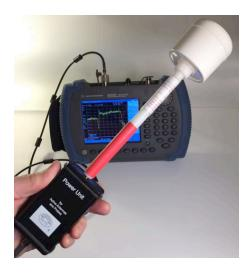
Active broadband isotropic antenna OFA-G for selective RF spectrum monitoring and field strength measurements. Antenna head has 3 internal orthogonal antennas. Signals from each antenna are combined to allow output signal to be proportional to the absolute value of the field strength regardless of the field direction.
