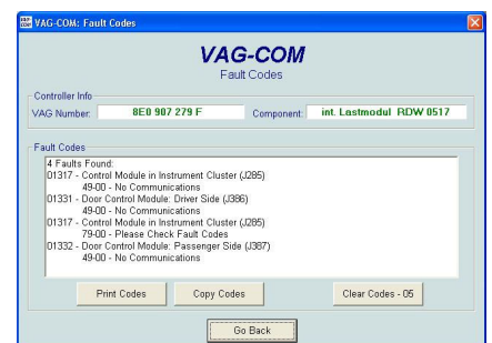
Reading out fault memory via the CAN diagnose bus
