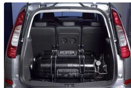
Additional fuel tank in the trunk of a fuel cell test car
