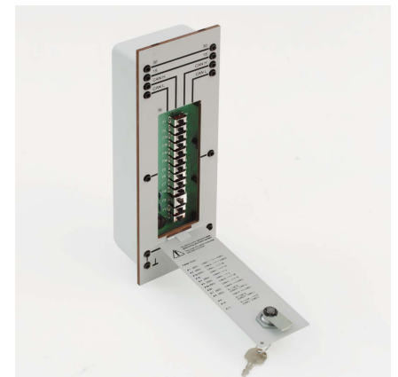
CAN bus fault simulator, 739 585
