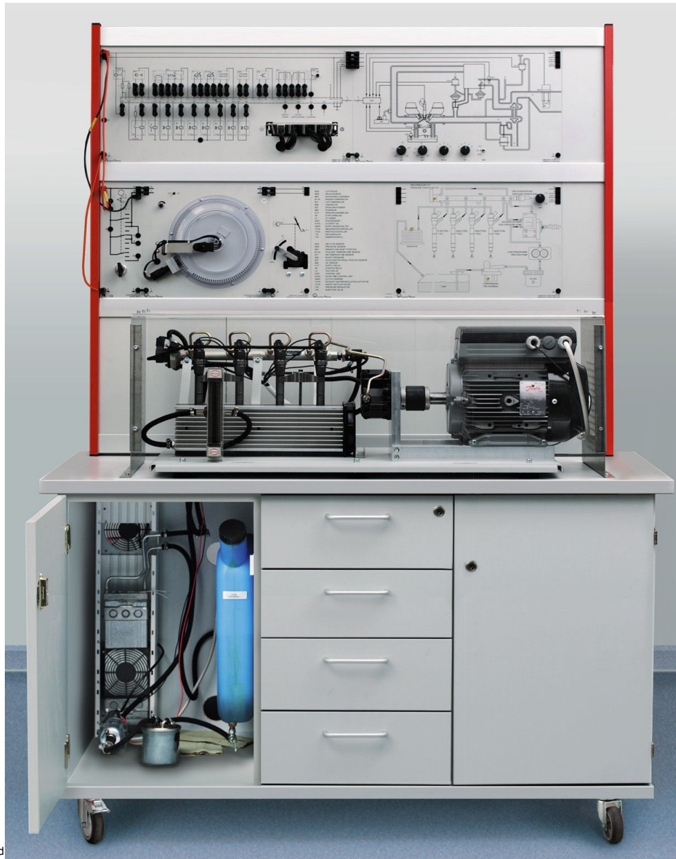
Complete common rail experiment stand with hydraulic components and fuel circuit
