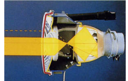
Structure of a polyellipsoid headlamp
