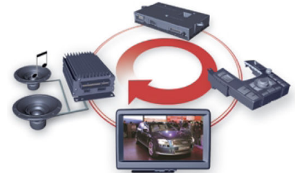
Audio/Video data transfer in MOST ring
