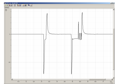
CASSY recording of an injector signal, left the pre-injection pulse and right the main injection
