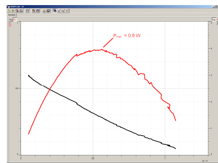
Stack voltage and power as a function of current, recorded with CASSY
