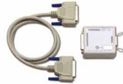
This is a terminal unit for converting a 25-pin SIGNAL I/O connector of TOS5300/5301/5302/5200 to a 14-pin SIGNAL I/O connector of TOS5050A/5051A. By connecting via this product, the external control performed with TOS5050A/5051A can be performed with TOS5300/5301/5302 at the same time.
