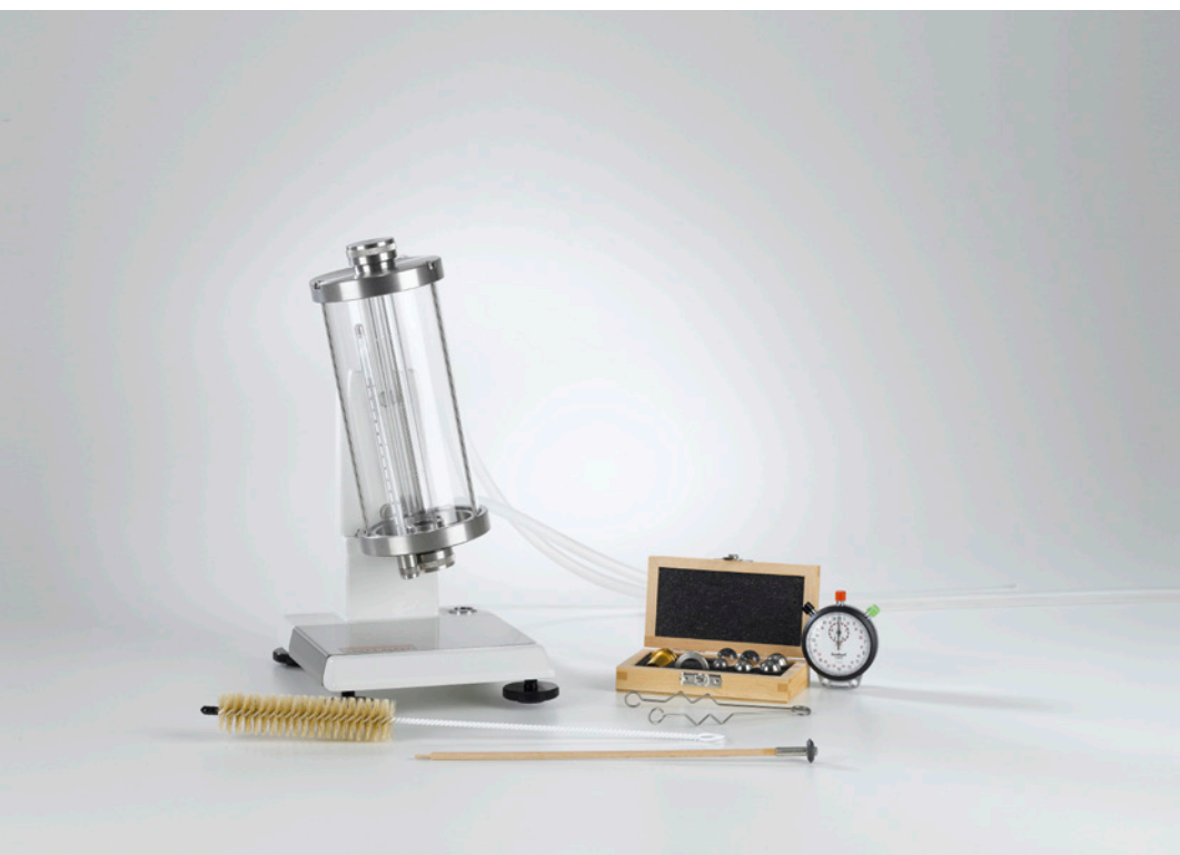
Determination of viscosity with the falling ball viscometer according to Höppler (C3.1.2.1)
