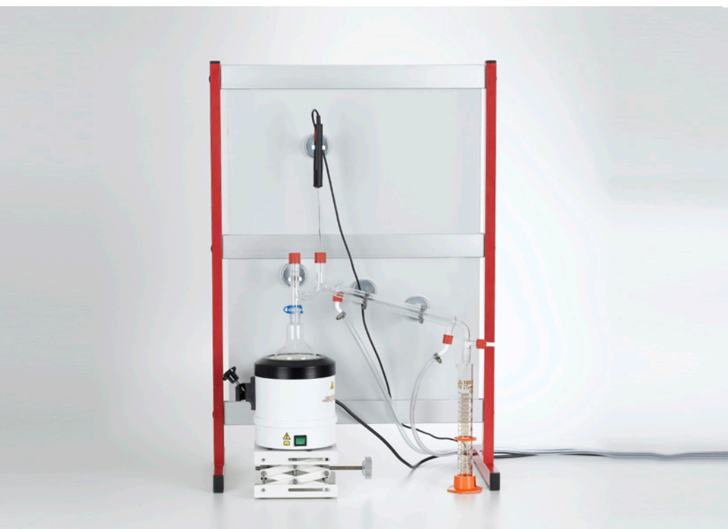
Boiling range distribution of petrol (C2.3.3.1)
