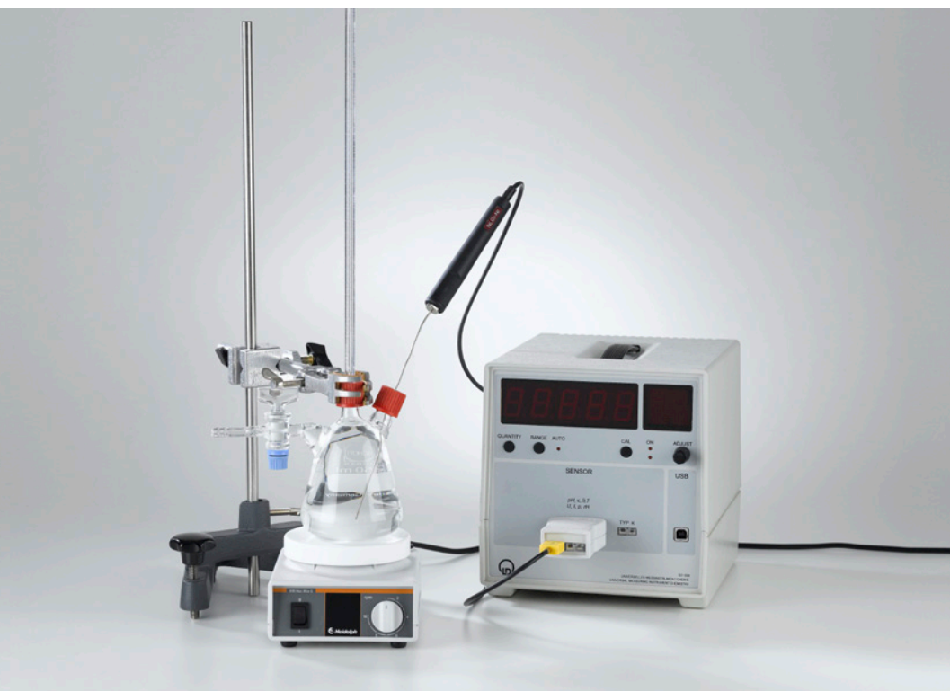
Thermal anomaly of water (C1.3.3.1)
