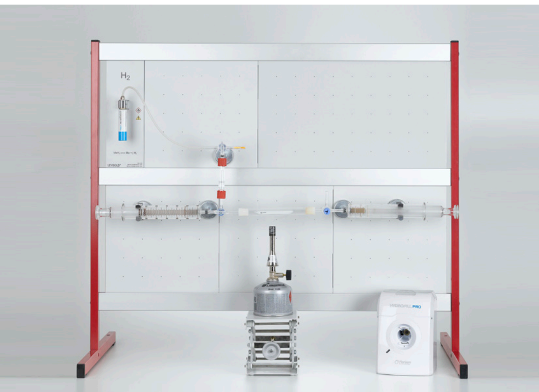
Synthesis of ammonia by the Haber-Bosch process (C5.1.1.2)
