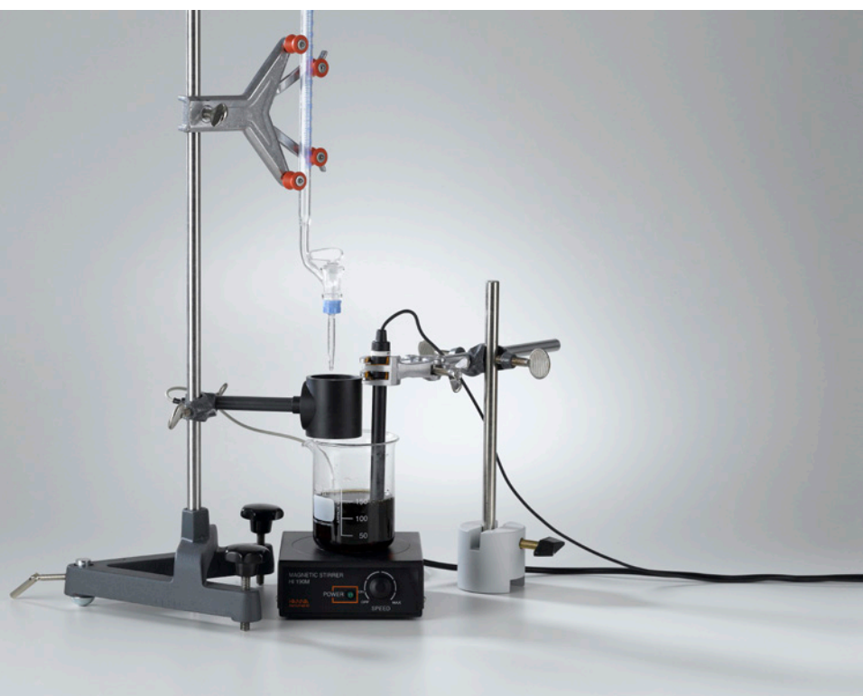
Determination of acid concentration by titration with drop counter (C3.5.1.1)
