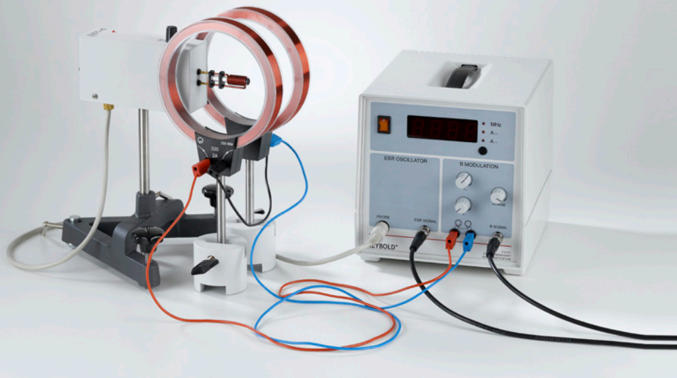
Electron spin resonance on DPPH (C3.4.4.1)
