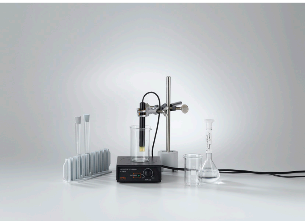
Enzymatics: Splitting urea with urease (C6.1.2.1)
