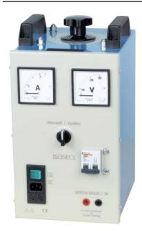
Adjustable from 0 to 230V in DC or AC, this power supply delivers a constant current of 3A. Protected by a thermal-magnetic circuit breaker, the safety of users is ensured by the separation of circuits.
