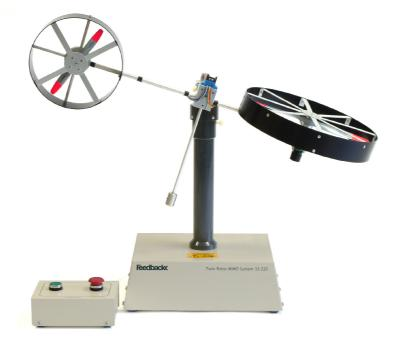
The Twin Rotor System demonstrates the principles of a non-linear MIMO (Multiple Input Multiple Output) system, with significant cross-coupling. Its behaviour resembles a helicopter, but the angle of attack of the rotors is fixed and the aerodynamic forces are controlled by varying the speeds of the motors.
