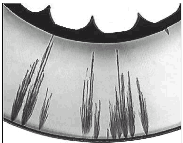
Water trees in a 0,5 mm slice of a 24 kV XLPE cable with tape and graphite insulation screen.
