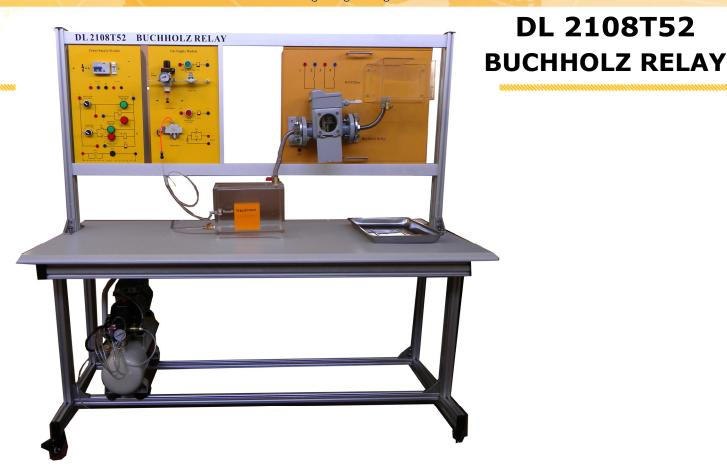
This trainer has the objective of studying the characteristics of a Buchholz Relay and in a more general way the identification and the features relevant to the failure in a oil circuit due to the presence of gas.
