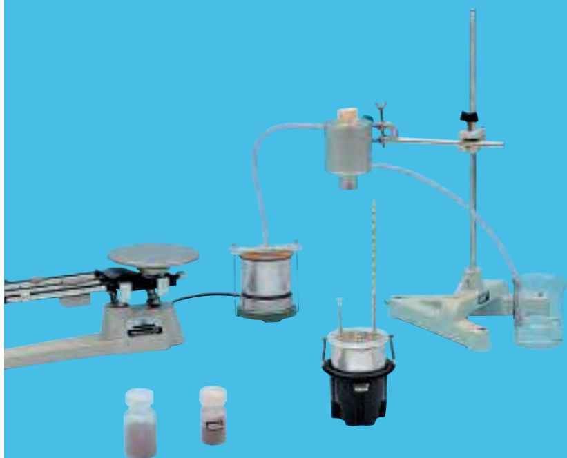
Determining the specific heat of solids (P2.3.2.1_a)
