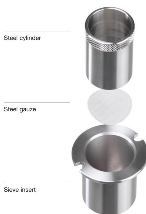
3-part stainless steel sample holder
