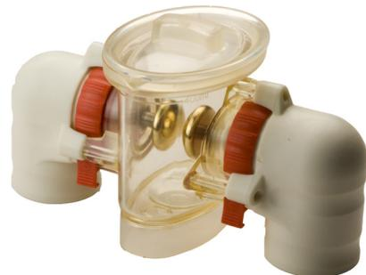
400 ml vessel assembly (with electrodes fitted)
