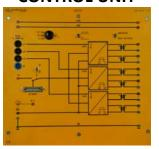
Trigger pulse generator for the triggering of thyristors or triacs in the single-phase and threephase rectifier and inverter circuits as well as in AC controllers. Possibility of analog control or digital control through interface.
