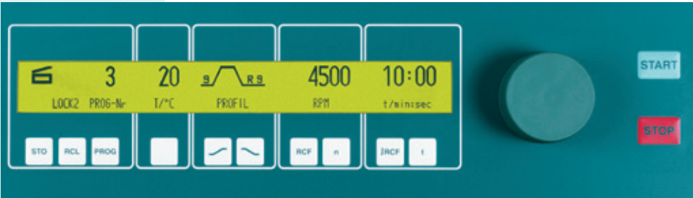
ROTO SILENTA 630 RS control panel: Entry of the parameters is exact, fast and easy with selector keys on the foil keypad and the adjusting knob.
