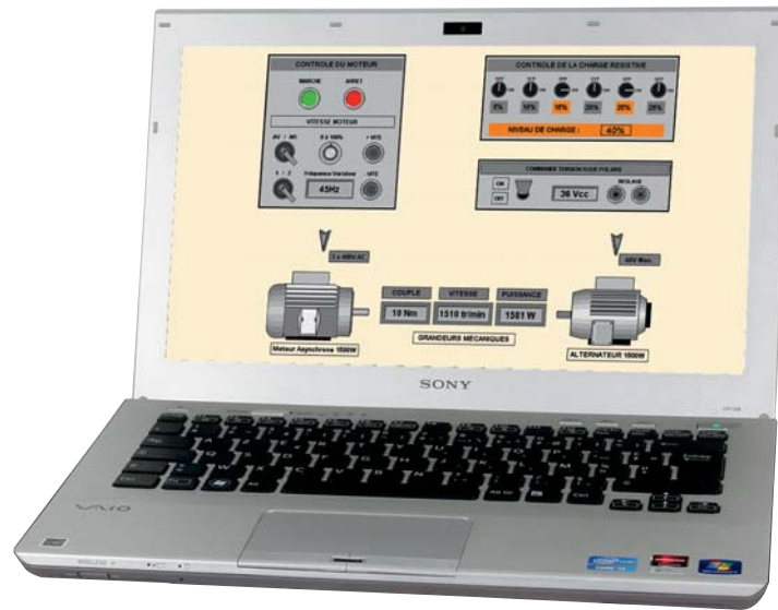
EXAMPLE OF SUPERVISION ON PC OF MTD5 MODEL MOTOR + THREE-PHASE ALTERNATOR
