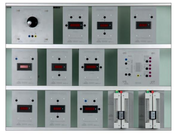
QUICK-G is a set of modules (H-250mm) for studying a compensated single-phase transformer 230V with three secondary windings.
