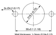
Wall thickness: 1-3mm (0.04-0.12) Mounting torque: 1.5Nm
