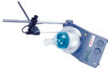
MS-H-Pro+ with PT1000 and reaction block
