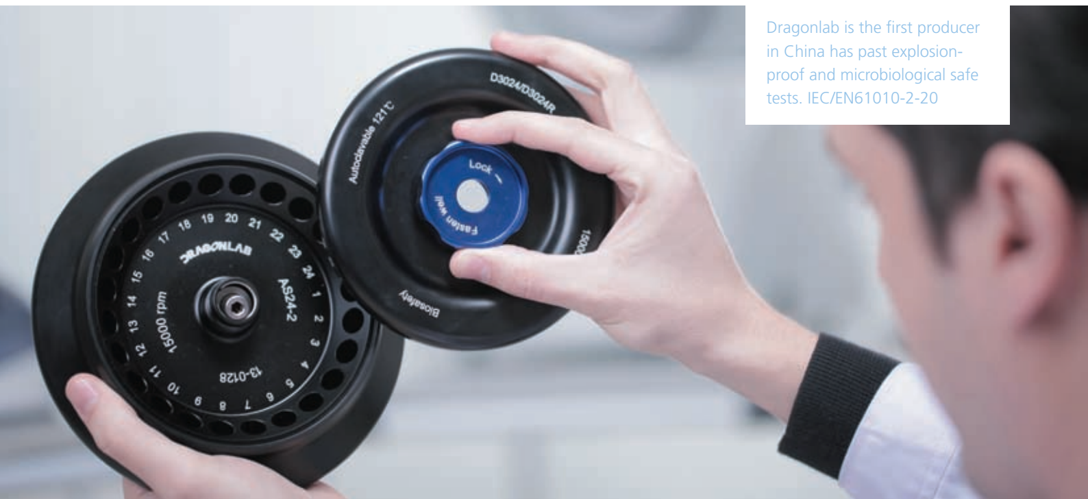
Seals within the aluminum alloy rotor
