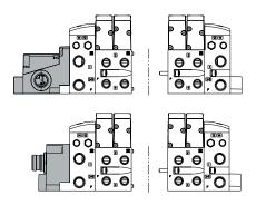
Manifold assembly with G3 Electronics & Discrete I/O (see page 13 and X021-26)
