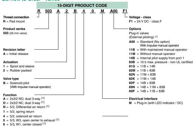
Used external spool valves (internal/external supply configurated in the end plate kits).
