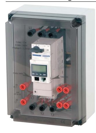
**CONTYS** from mecatronics is a motor starter which combines mechanical, electrotechnical and electronic technologies. It is designed to be used for directly starting up motors of up to 3kW. This compact device combines power functions (disconnecting switch, commutation) and control functions (protection).
